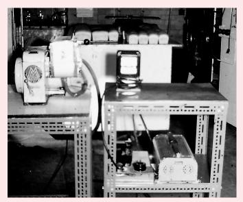
mixers the BBIRA team found that though the crumb cell structure varied from one mixer to another, the optimum work input (in terms of bread volume) remained essentially the same. They calculated energy levels in the dough and found that the optimum for the range of flours available at that time was 0.4 h.p. (horse-power) min/lb, equivalent to 5 Wh/lb, 11 Wh/kg or 42 kJ/kg of dough in the mixer.
